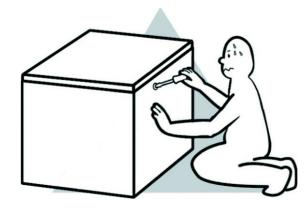
**DO NOT** fully tighten screws (leave slightly loose). When the item is fully assembled tighten the screws - but do not over tighten.
