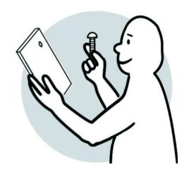
Separate and identify each component from the hardware pack and rest each one in its proper location before fastening.
